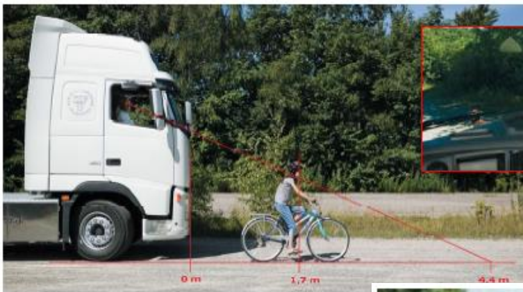
Figure 4 Distance in front of vehicle, necessary for cyclist to be seen directly by driver and the view from the cab, showing little leeway for error
