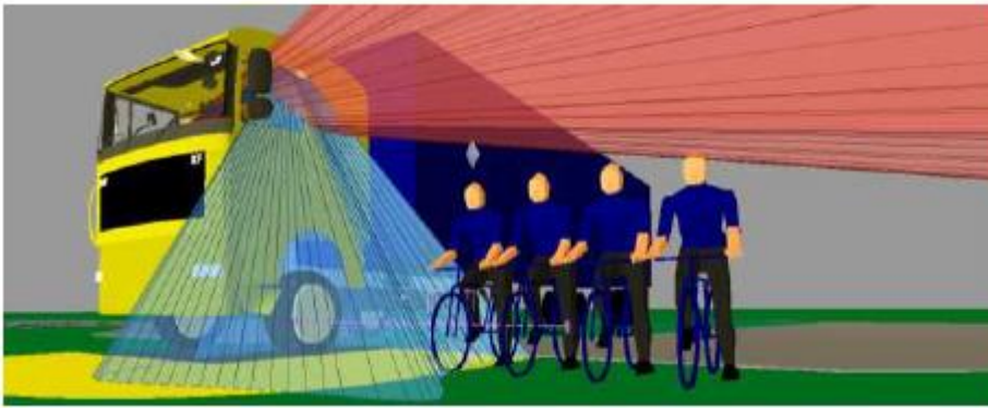
Figure 7 Blind Spot between the Class IV and V mirrors and window Direct Vision
