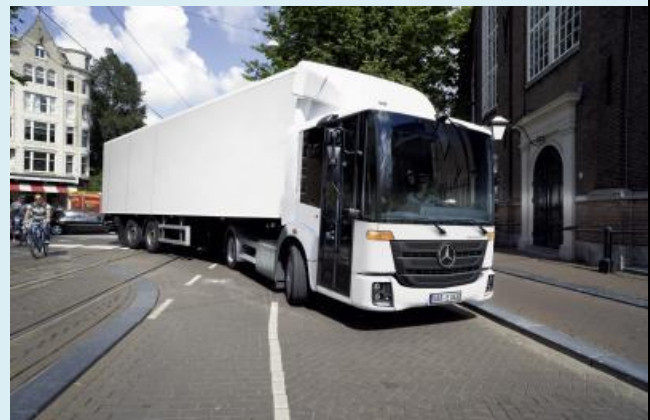
Figure 10 such as this prototype Mercedes Benz cab. Low driving position, large windscreen and fully glazed doors.
