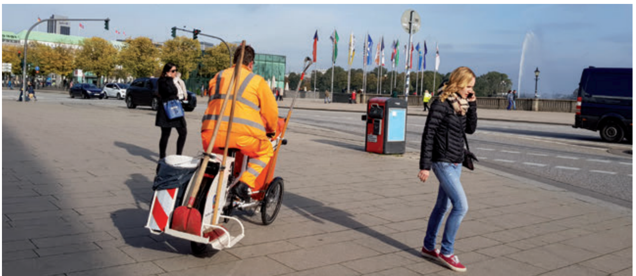
Picture 4: The Veleon has a small turning radius beneficial in highly frequented areas, but has higher maintenance costs, SRH
